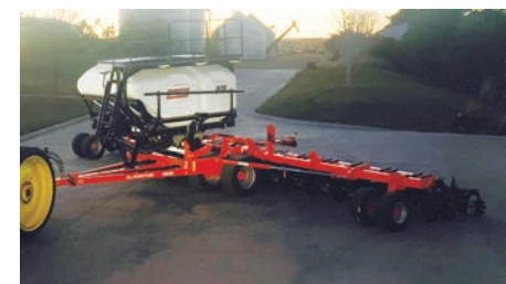
ST-10, 10 ton single tank metering mounted directly on application tool bar.
