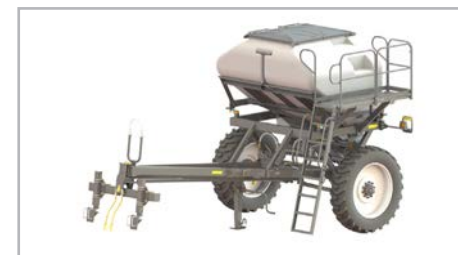
ST-6, 6 ton single tank metering mounted on Salford PATHFINDER.
